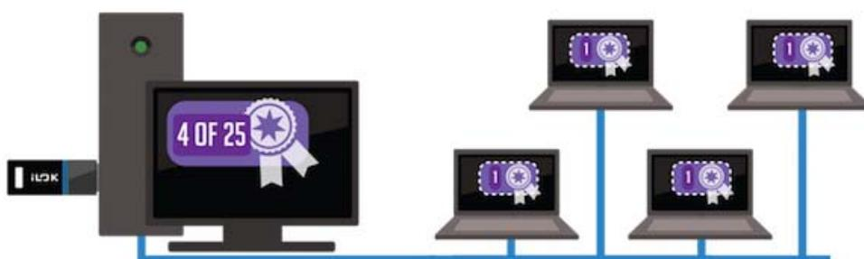
Illustration showing a license server activating 4 copies (seats) of an application over a local network using a sharable license that can activate up to 25 seats.
